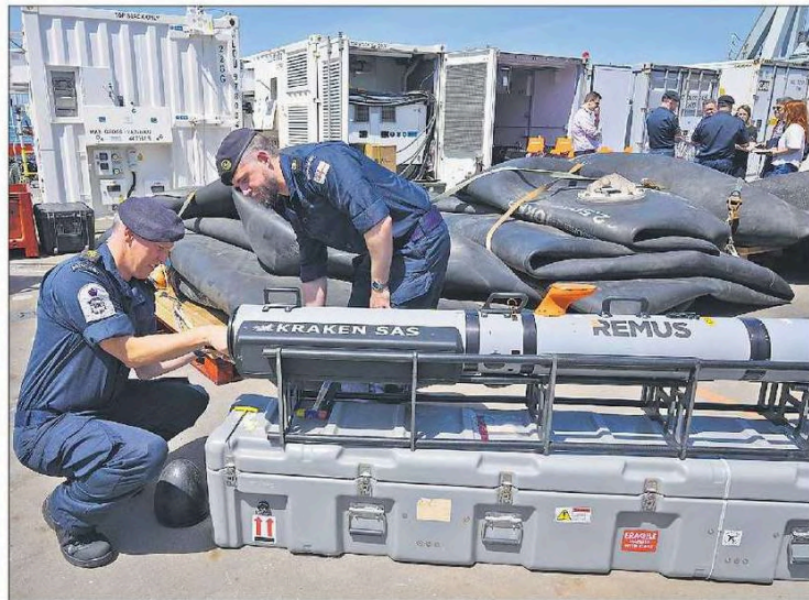
Autonomous vehicles with sonar that can detect and identify mines, on RFA Lyme Bay on Friday. AP
